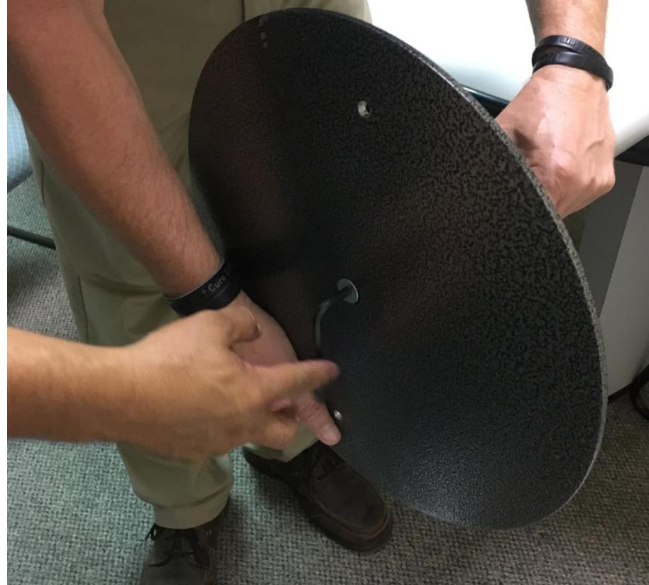
Place base on pole, be sure the holes are perpendicular to where the horizontal bar will be. It's easier if someone can hold pole and base while the other lines up the screw and tightens.
