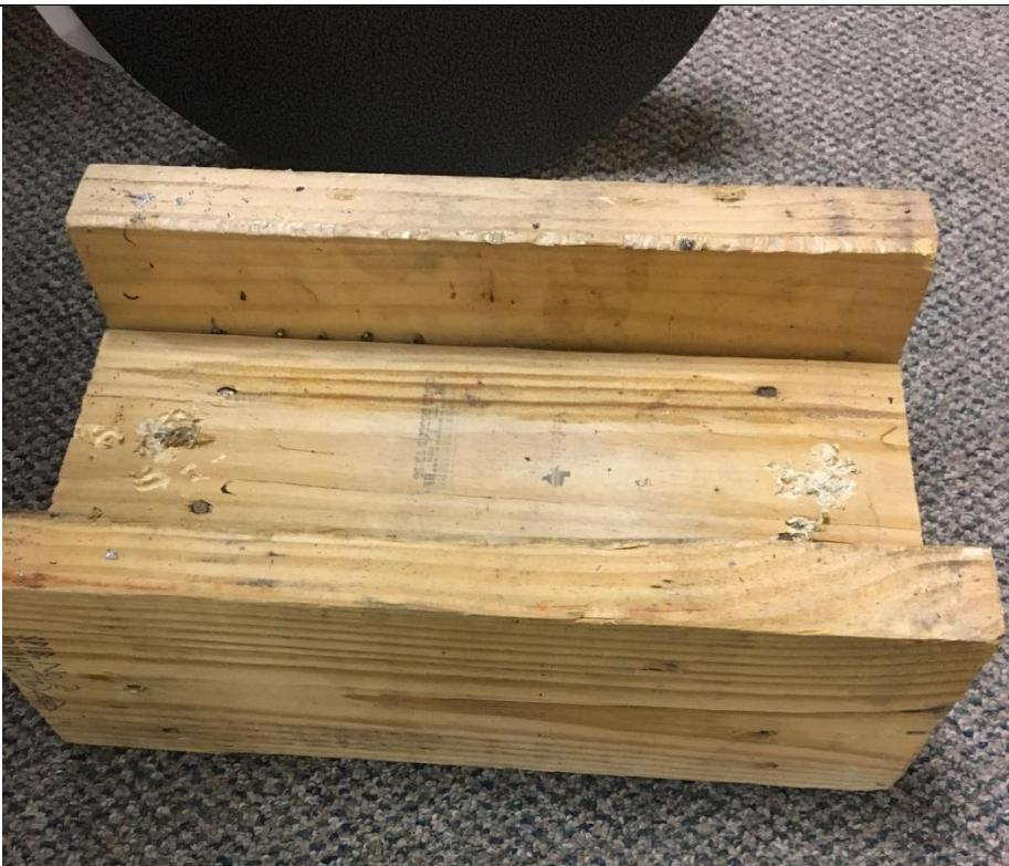
Build a small structure using 2x6 studs as shown in the picture to give you room for the drill.
