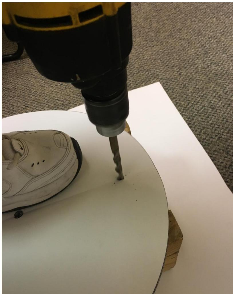
Place base and pattern on wood structure. You can use your foot to hold pattern in place. Drill both marked circles.
